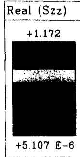
Fig. 3. Recalculated normal stress at the end surface of the cylinder (at z = 0 ) on the real part of the deformed configuration for Case 2 (Patch Loading). The localized normal displacement can be seen ( \Omega = 2, \nu = 0.3317 ). The black mesh represents the undeformed configuration.
